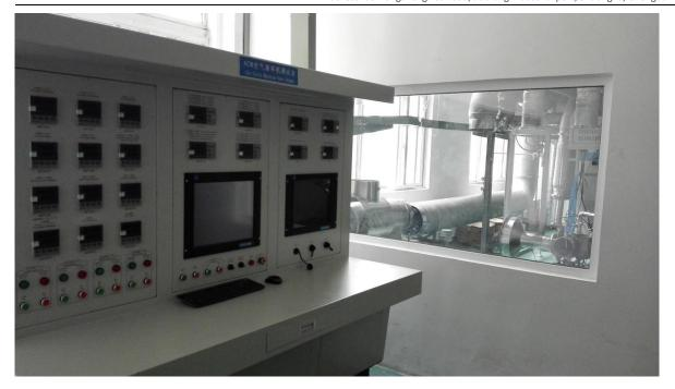
ACM air circulator test system is mainly used to test ACM performance under no-load and different air pressure. The main test contents include external leak test, functional test and electrical connection test, which can measure ACM speed and test of inlet and outlet air pressure, temperature, rotating shaft vibration peak value and shaft vibration when no load.
